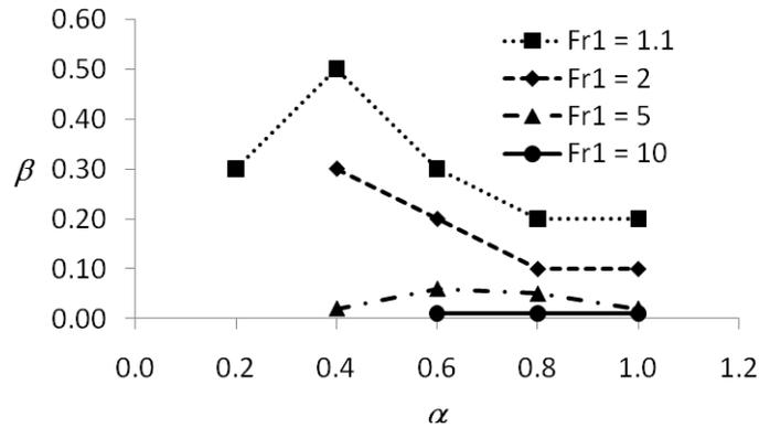
Fig.2: Maximal admissible value of  $\beta$  as a function of  $\alpha$  and  $Fr_1$  (RSW1)
