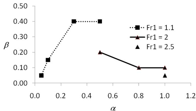
Fig.11: Maximal admissible value of  $\beta$  as a function of  $\alpha$  and  $Fr_1$  (RSW1)
