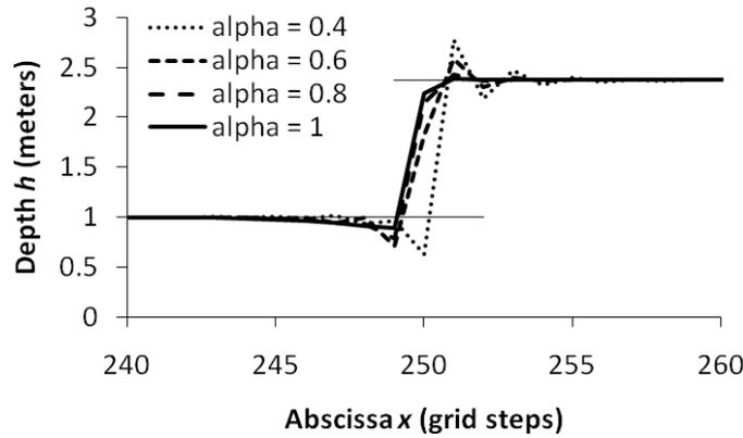
Fig.4: Distribution of depth for  $Fr_1 = 2$  (RSW1)
