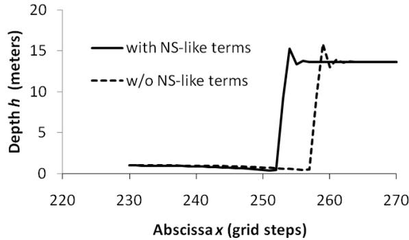
Fig.8: Distribution of depth for  $Fr_1 = 10$ ,  $\alpha = 0.6$  (RSW1, influence of NS-like regularizing terms)
