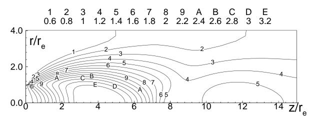
Figure 24: Iso-Mach lines. Regular reflection.  $Ma_e = 1.1, Kn_e = 0.01.$
