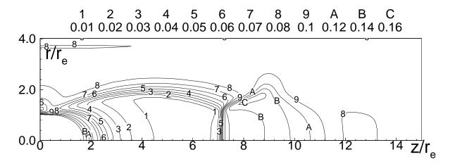
Figure 25: Isobar lines. Mach reflection.  $Ma_e = 1.1, Kn_e = 0.002.$
