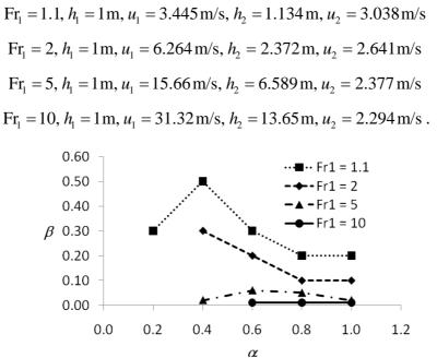
Fig.2: Maximal admissible value of  $\beta$  as a function of  $\alpha$  and Fr<sub>1</sub> (RSW1)
