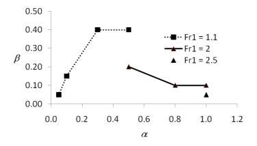
Fig.11: Maximal admissible value of  $\beta$  as a function of  $\alpha$  and Fr<sub>1</sub> (RSW1)
