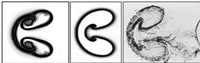
Fig. 5 - Helium bubble. Bubble form at time moment  $t = 1.342 \cdot 10^{-3}$ . Our results (left), results from Quirk J, Karni S, 1996 (middle) and experiment from Haas JF, Sturtevant B, 1987 (right)
