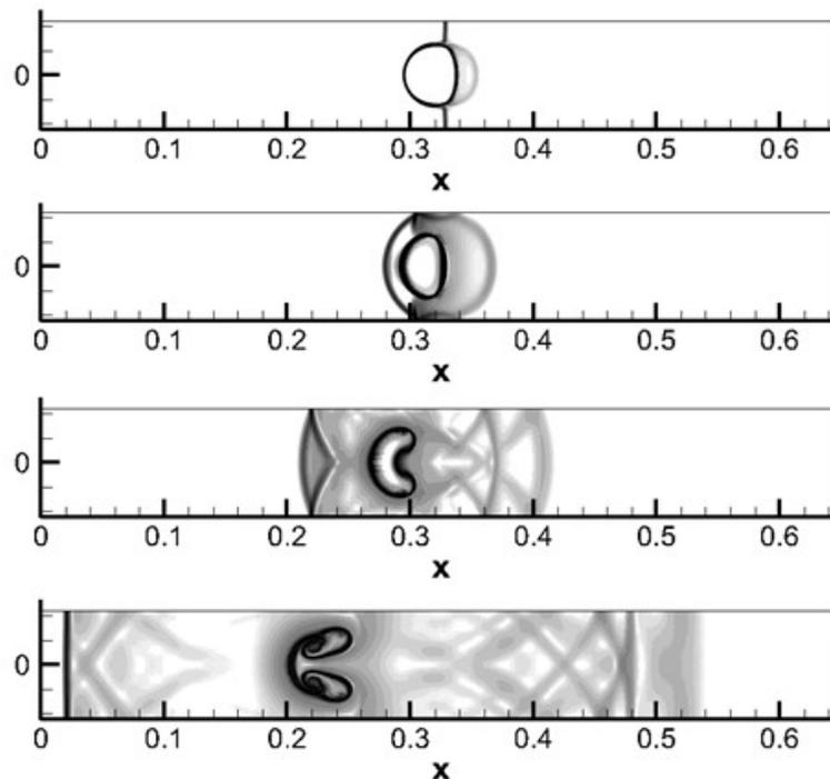
Fig. 4 - Helium bubble. Numerical schlieren images at successive time moments (from top to bottom):
