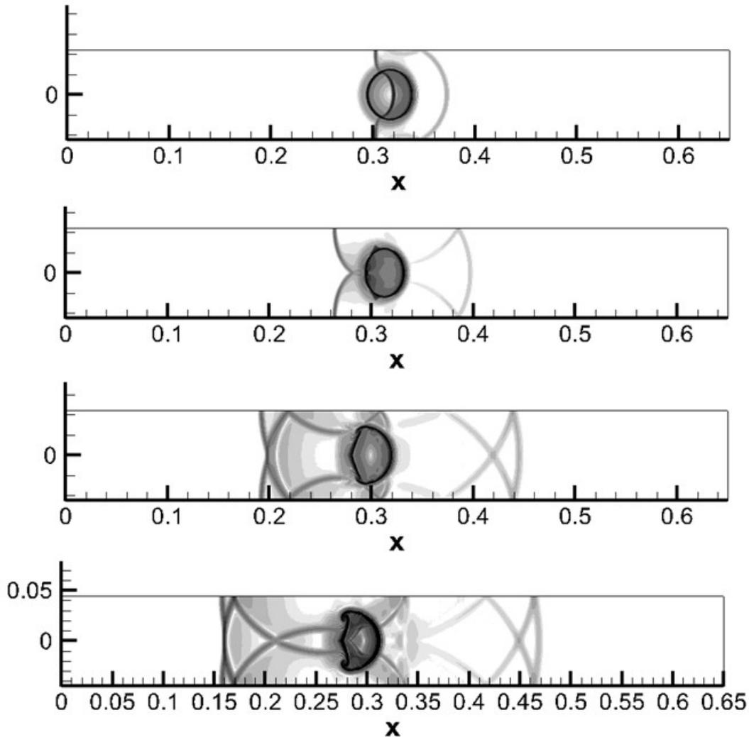
Fig. 2 - R22 bubble. Numerical schlieren images at successive time moments (from top to bottom):
