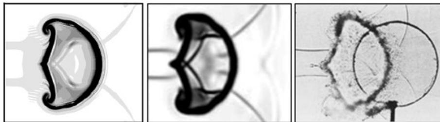
Fig. 3 - R22 bubble. Bubble form at the time moment  $t = 1.1 \cdot 10^{-3}$ . Our results (left), results from Quirk J., Karni S., 1996 (middle) and experiment from Haas JF, Sturtevant B., 1987 (right)
